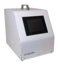
A touch-screen display and intuitive user interface allows measurement parameters to be configured and sampling to begin within a matter of minutes. The on-board computer allows unattended operation, data storage and processing. This product satisfies the long-standing need for a research-grade instrument that is portable and straightforward to integrate into application-specific testing and research.
